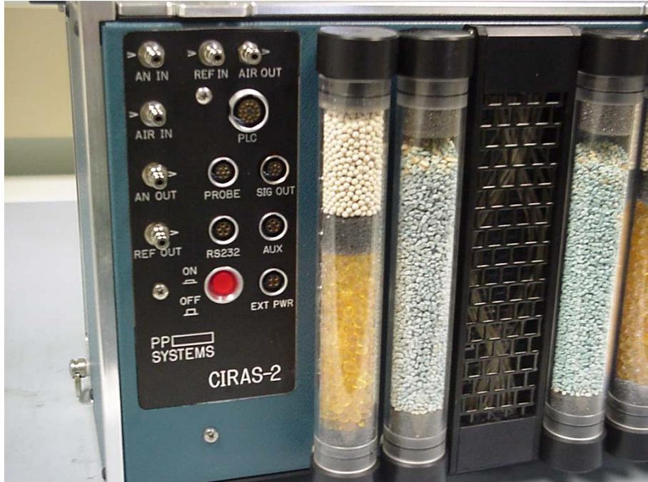
Figure 1 CIRAS-2 Electrical and Air Connections
