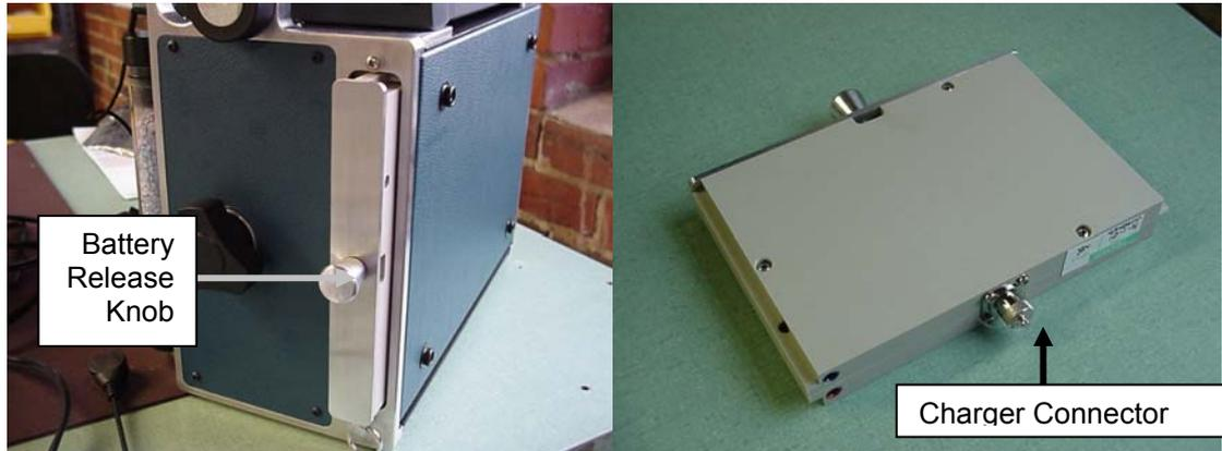
**Figure 17 Charging Batteries**
