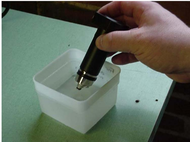
**Figure 13 Testing CO<sub>2</sub> Cartridge Flow**
