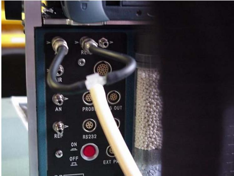
**Figure 7 Tubing Connections to Test CIRAS-2 as an IRGA Only.**
