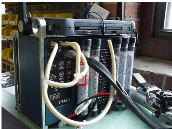
**Figure 8 Electrical and Pneumatic Connections**
