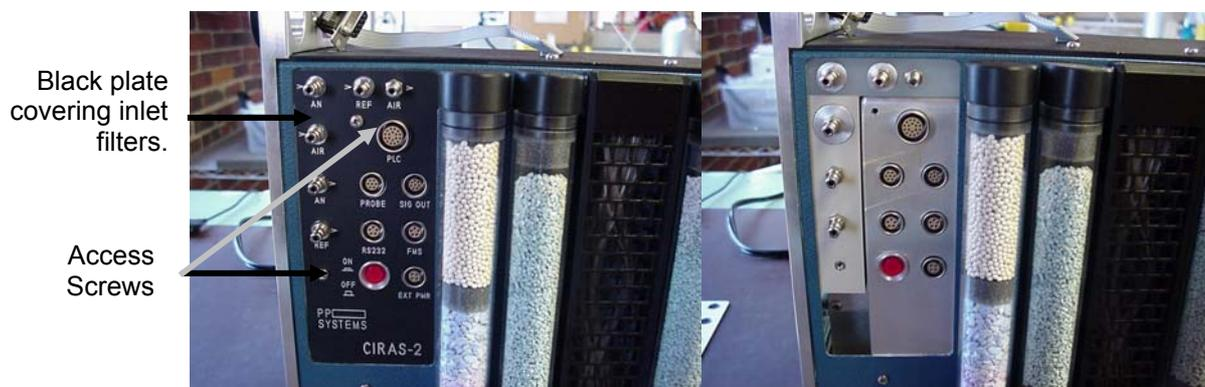
**Figure 14 Removal of Back Plate to access Filters**
