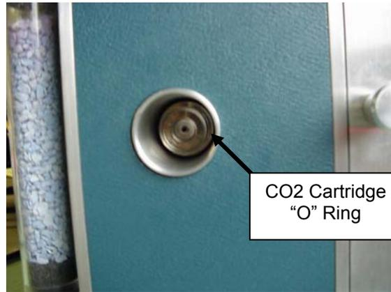
**Figure 12 CO<sub>2</sub> Cartridge "O" Ring**
